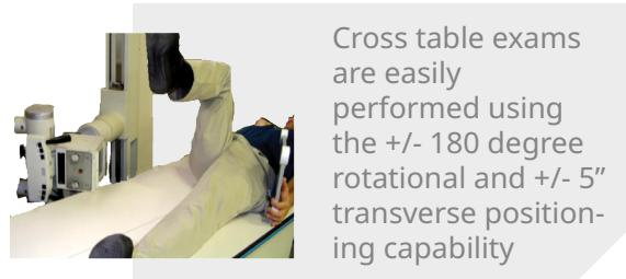
Cross table exams are easily performed using the +/- 180 degree rotational and +/- 5" transverse positioning capability
