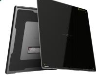
Rayence innovations in manufacturing have allowed us to create a new generation of Low Dose Cesium Iodine wireless detectors to meet the needs of all applications with superior image quality at a substantially lower dose.
